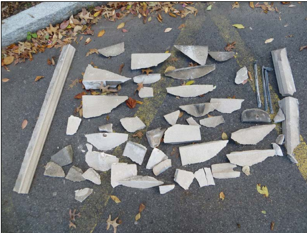
Photograph 6: MPS removed several pieces of stone from the building that were ready to fall. This picture does not include the multiple pieces of stone that have already fallen to the ground. The falling stone pieces prompted the installation of the fencing and overhead protection.
