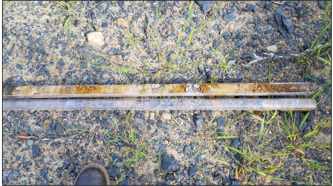
Photo 5. View of orange/brown silt encountered just before refusal in SB-030. Although the depth and thickness varied, the material was consistent wherever refusal was encountered. Photo taken August 2017.
