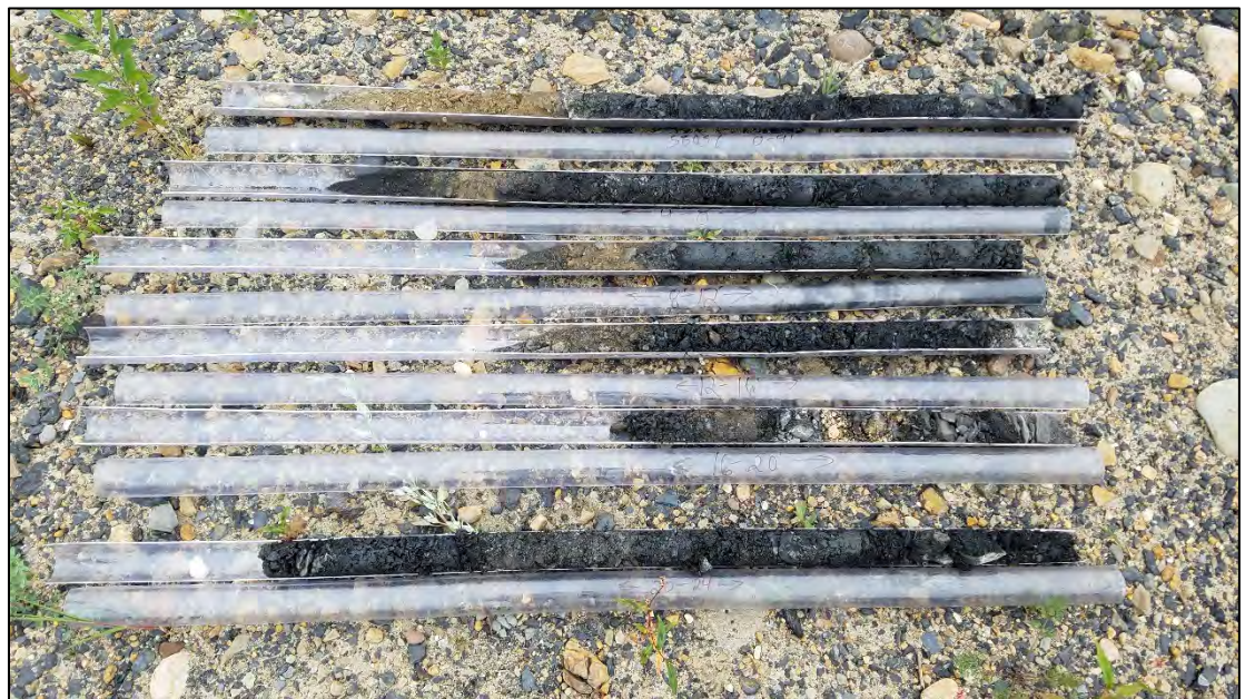
Photo 4. View of sample sleeves from SB-037. Majority of recovery was coal material which was typical of all borings.
